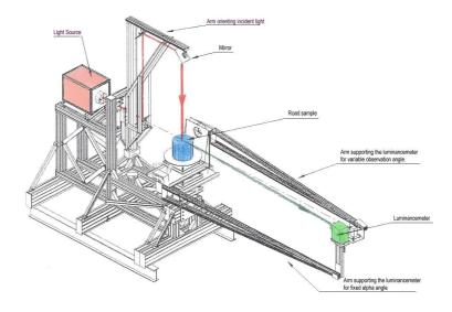
In this context, Schréder launched 3 years ago, in collaboration with the University of Liège, a research project called Memphis which aimed to improve the knowledge of road surfaces and overall to develop equipment capable of measuring the reflection characteristics of road surfaces on site.
