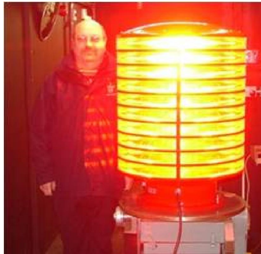
Figure 3 Ten-tier Red LED Omnidirectional Light giving around 35,000cd
