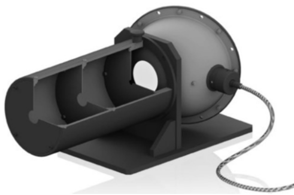
Figure 3 – Realization of the alternative method with the PTFE integrating sphere and a tube with all necessary apertures for the BLH measurements.
