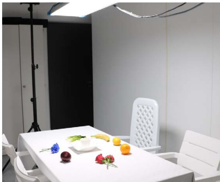
Figure 1 – Arrangement of seven coloured objects in the psychophysical experiment illuminated by the LED light engine. The 8 th object was the subject's own hand (not depicted)
