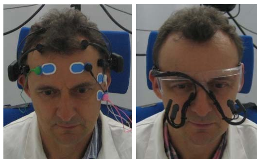
Figure 3 – Subject equipped with EMG, EEG and ECG (left) and with eye tracker and ECG (right)
