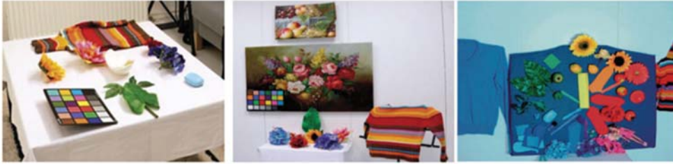
Figure 1 - Colour samples in visual tests under different CCTs, chroma and Illuminances
