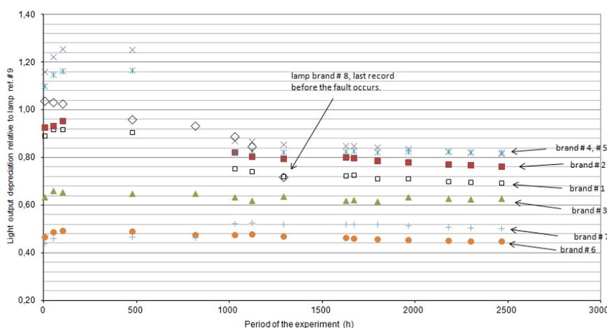
**Figure 8 – The light output results of six different WLEDi lamp brand (base E-27 type) used in for the long term experiment and sampled after thermal stabilization of 5 minutes**
