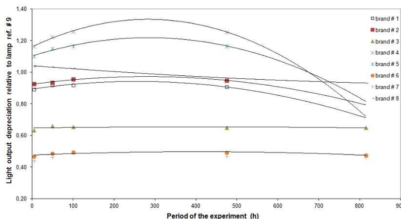
**Figure 7 – The light output results from six different WLEDi lamp brand and eight samples (base E-27 type) during the first 815 h of the long term experiment**
