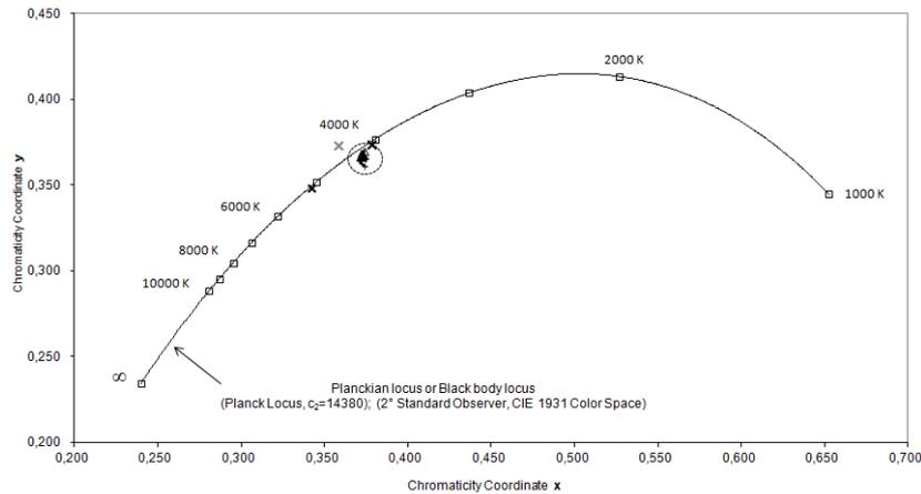
**Figure 4 – The CIE 1931 (x, y) space diagram with chromaticity coordinates sampled from WLEDi equipment (the points circumscribed by the dashed line were sampled from luminaires currently installed at CUASO-USP and the three cross-type notations indicate other WLEDi equipment (BURINI JUNIOR, E. C. et al. 2015a)**
