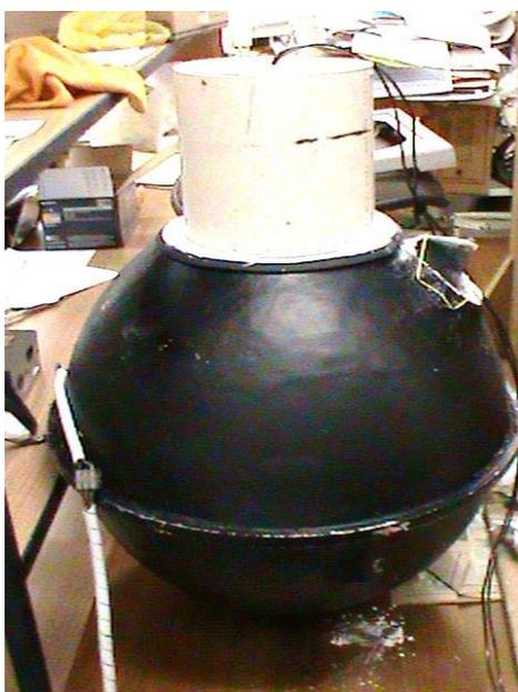
**Figure 2 – The integrating photometer (at bottom: sphere in black colour) with the housing designed (cylinder in white colour) mounted on top, after February, 2019**
