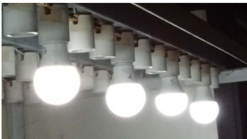
**Figure 3 – WLEDi lamps installed (base up position, E-27, 225 Vac) running at the test site**
