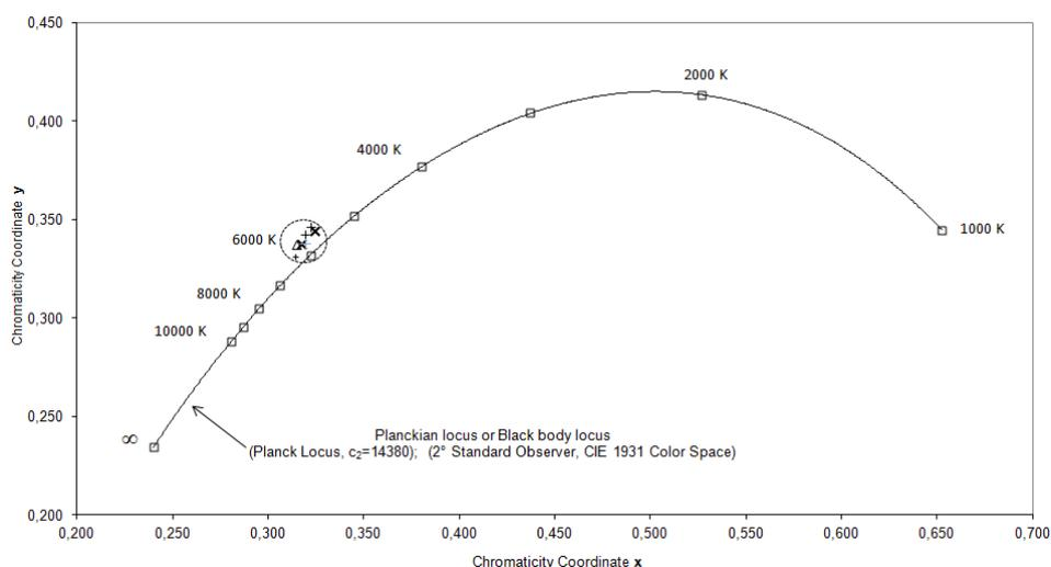
**Figure 6 – The CIE 1931 (x, y) space diagram with chromaticity coordinates from WLEDi lamps, (base E-27 type) used in for the long term experiment and sampled initially after thermal stabilization of 60 minutes (BURINI JUNIOR, E. C. et al. 2019a)**
