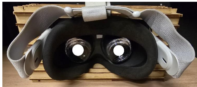
Figure 1 – The Meta Quest 2 HMD used in the experiment, with white circles representing a circular stimulus displayed to the observer.
