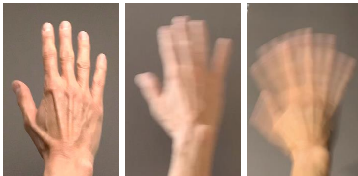
Figure 1 – Left: motionless hand, centre: the moving hand still appears as a single object, right: the fingers of the hand can be seen multiple times due to the stroboscopic effect.
